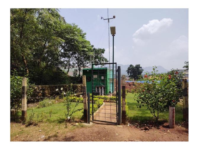
Online AAQMS installed at mines for continuous monitoring of parameters like CO , SO2, PM10, PM2.5 and NOx.
